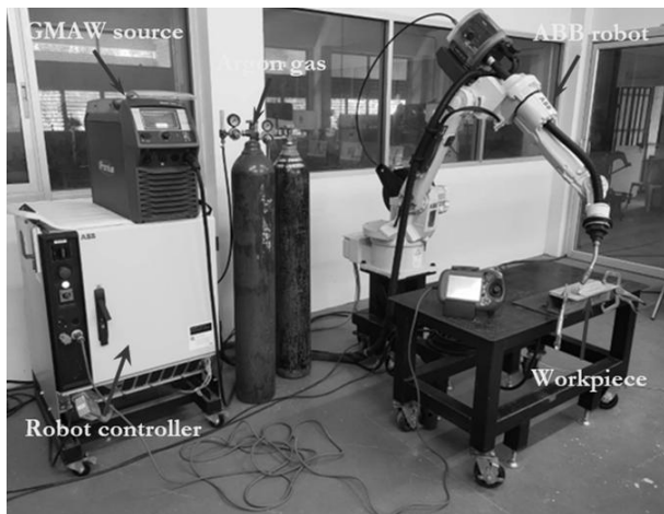
Fig. 1 Experimental setup of robotic GMAW-based additive manufacturing system for aluminum wire deposition
