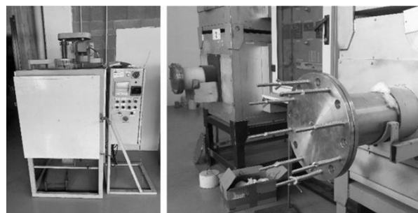
Fig. 3 Chamber furnace with circulation and tube furnace with metal muff
