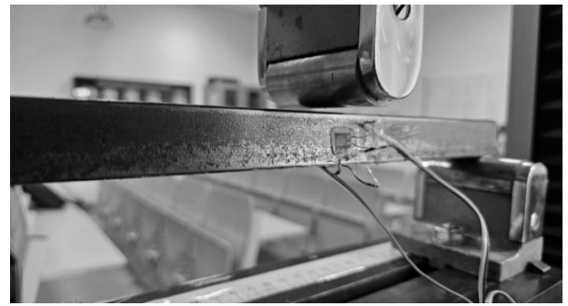
Fig. 2 Sample with a resistance strain gauge attached
