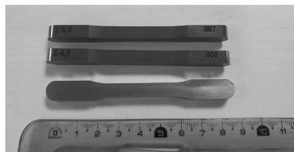
Fig. 1 Pressed samples for testing mechanical properties
