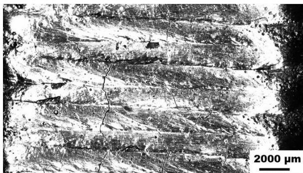
Fig. 14 The surface of a weld cladding coating made from high hardness powder 10.16.6 on a layer of Inconel 625 – cracks appeared in the weld cladding coating
