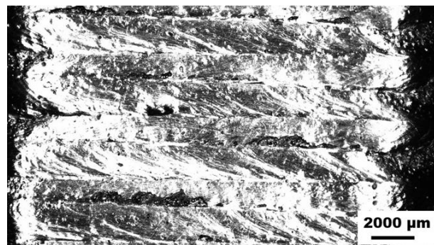
Fig. 15 The surface of a weld cladding coating made from medium hardness powder 10.12.6 on a layer of Inconel 625 – the weld cladding coating was free of cracks
