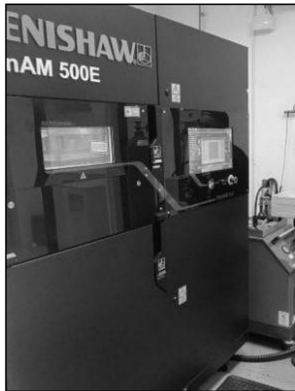
Fig. 1 SLM Machine Type RenAM 500E
