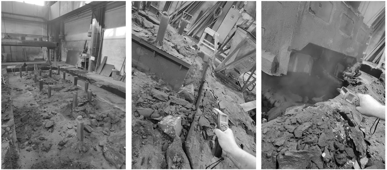
Fig. 9 Temperature measurement of the casting using a pyrometer immediately after its removal from the sand mould (pit face)
