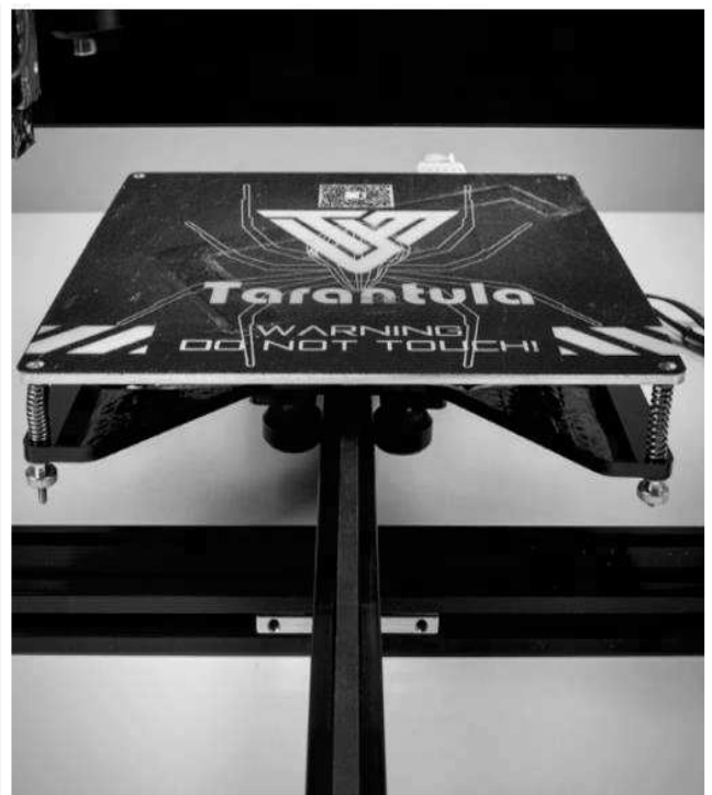
Fig. 1 Commercially available TEVO Tarantula device selected for optimization
