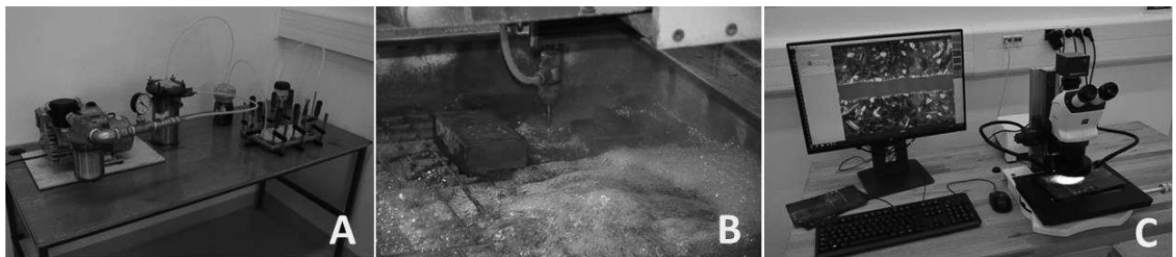
Fig. 3 Testing process: A: production of composite material by vacuum infusion, B: cutting of composite material by CNC cutting machine AWJ CT 0806 with different traverse speed of cutting head, C: evaluation of cut by means of optical analysis.
