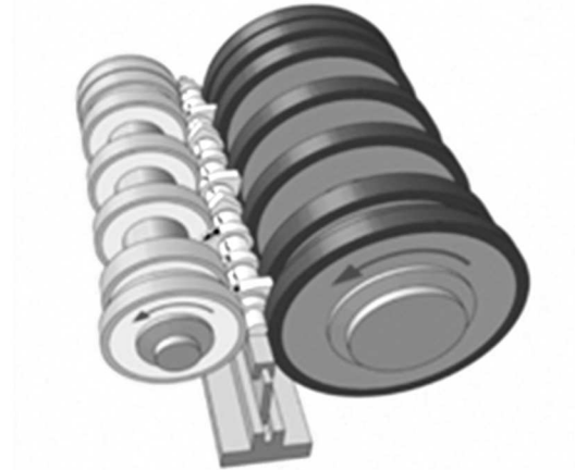
Fig. 1 Scheme of centreless groove grinding [8]
