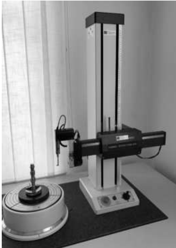
Fig. 7 Device for measuring of circularity - Hommel Tester Form T4004
