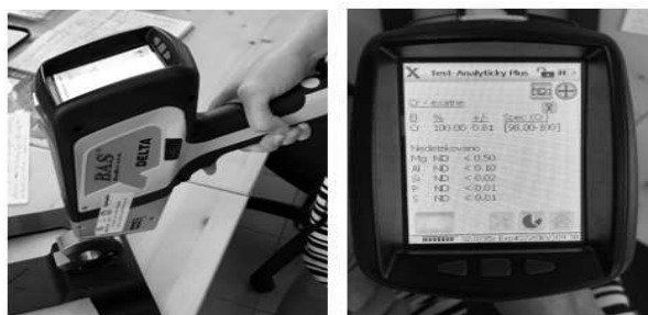
Fig. 3 DELTA optical spectrometry and chemical composition of chromium layer
